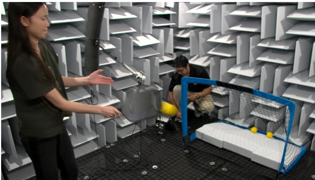
Figure 1: The sound pressure measurement set up for a pickleball paddle.
